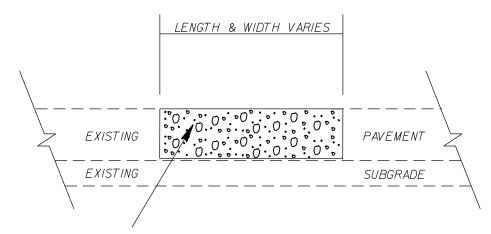
RATE IS VARIABLE AND SHALL BE AS DIRECTED BY THE ENGINEER. ASPHALT TYPE 119.0C SHALL BE PLACED.
